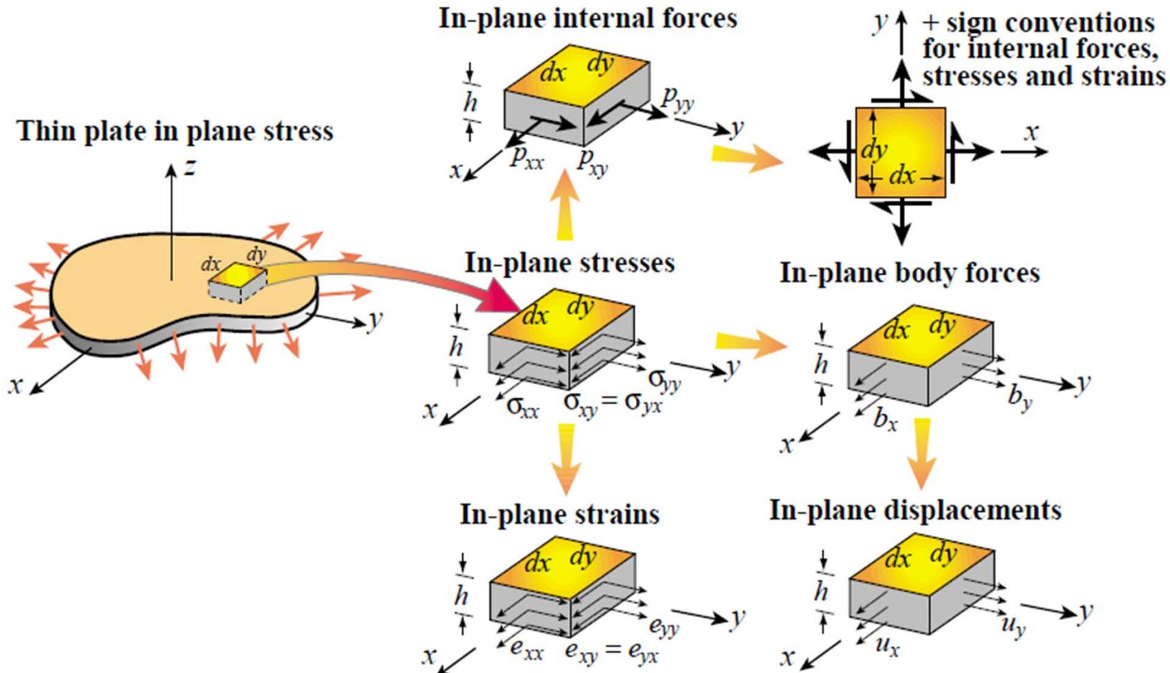
In-plane forces are obtained by stress integration through thickness.
