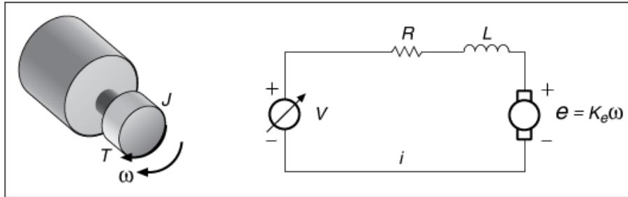
where  $V$  is the source voltage of the DC power supply.
