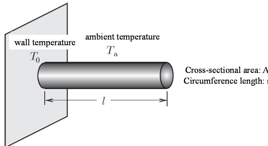
Diagram illustrating the 1D steady-state heat transfer problem. A cylindrical rod of length  $l$  is shown. At the left end ( $x = 0$ ), the wall temperature is  $T_0$ . At the right end ( $x = l$ ), the boundary condition is a heat flux  $Q_l$ , indicated by a normal vector pointing outwards. The ambient temperature is  $T_a$ . The cross-sectional area is  $A$  and the circumference length is  $s$ .
