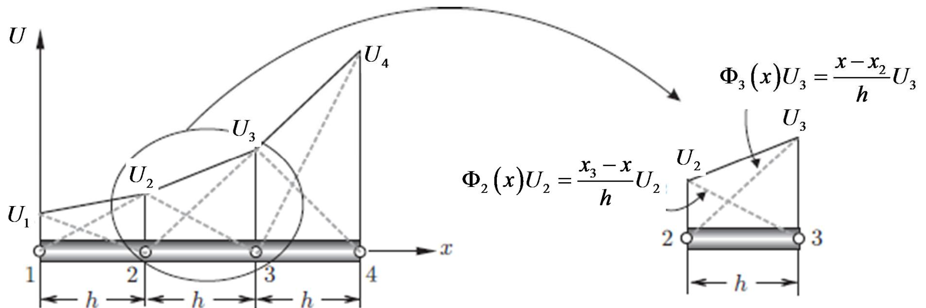
$$\begin{aligned} U(x) &= \Phi_2(x)U_2 + \Phi_3(x)U_3 \\ &= \frac{x_3 - x}{h}U_2 + \frac{x - x_2}{h}U_3 \quad (x_2 \leq x \leq x_3) \end{aligned}$$
