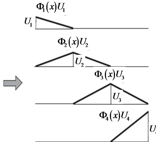
$$\begin{aligned} U(x) &= \Phi_1(x)U_1 + \Phi_2(x)U_2 + \Phi_3(x)U_3 + \Phi_4(x)U_4 \\ &= \sum_{i=1}^4 \Phi_i(x) \underbrace{U_i}_{\text{temperature @ node } i} \end{aligned}$$
