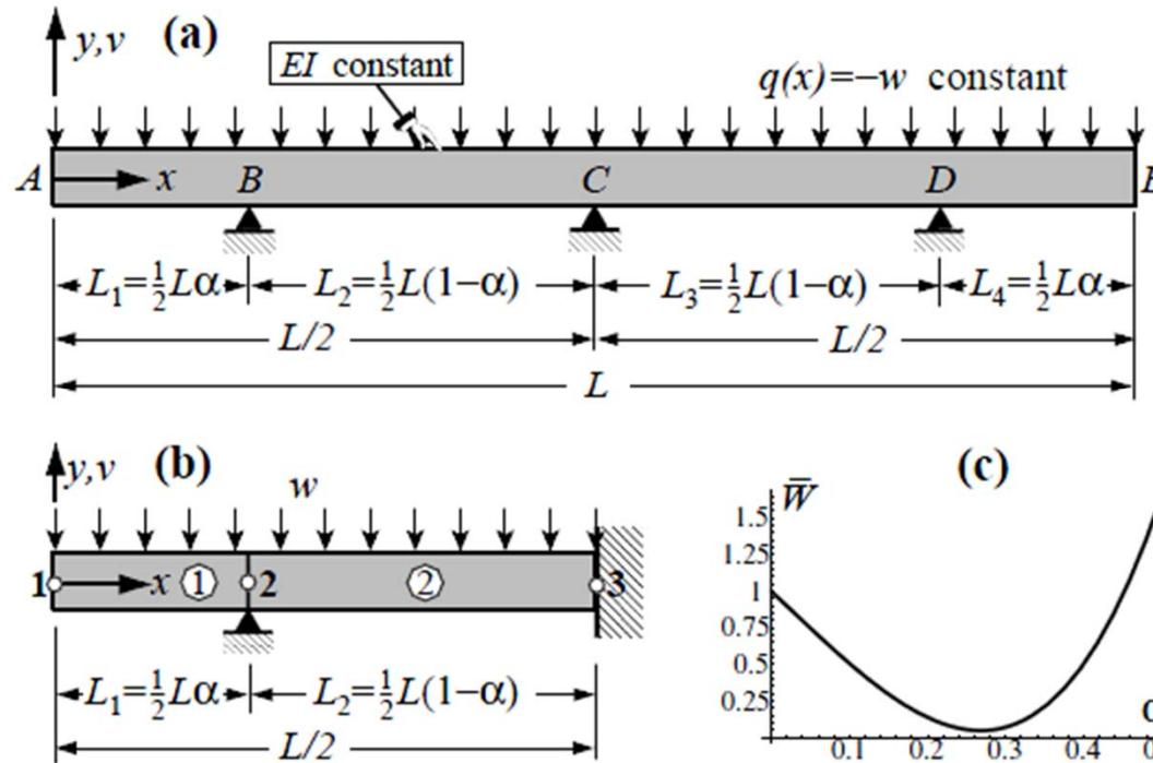
$$\text{best } \alpha \rightarrow \begin{cases} \text{Minimum external energy: } W(\alpha) = \mathbf{f}^T \mathbf{u} \rightarrow dW/d\alpha = 0 \rightarrow \alpha \approx 0.27 \\ \text{Equal reactions: } R_B = R_C \rightarrow \alpha = 0.30546 \\ \text{Minimum relative deflection: } v_{ji}^{\max}(\alpha) = \max |v_j - v_i| \rightarrow \alpha = 0.26681 \\ \text{Minimum absolute moment: } M^{\max}(\alpha) = \max |M(x, \alpha)| \rightarrow \alpha = 0.25540 \end{cases}$$
