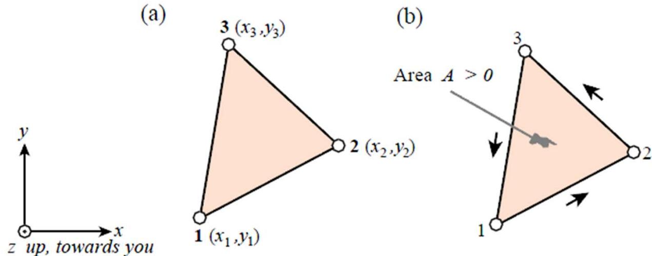
$$A_{023} = \frac{1}{2} |L_{02}| |L_{03}| \sin \theta = \frac{1}{2} L_{02} \times L_{03} = \frac{1}{2} \begin{vmatrix} x_2 & x_3 \\ y_2 & y_3 \end{vmatrix} = \frac{1}{2} (x_2 y_3 - x_3 y_2)$$
