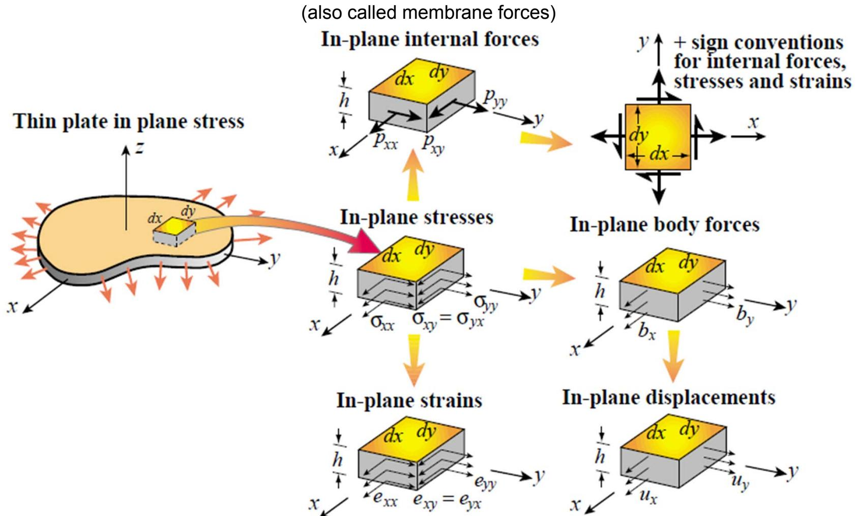
In-plane forces are obtained by stress integration through thickness.
