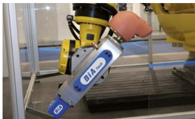
BHIA250-VC Launcher for FMH and Guided Head Impacts
