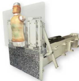
E-Liner BODYBLOCK for steering column- and airbag development tests
