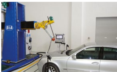
BIA Universal Impact Simulation Test System
