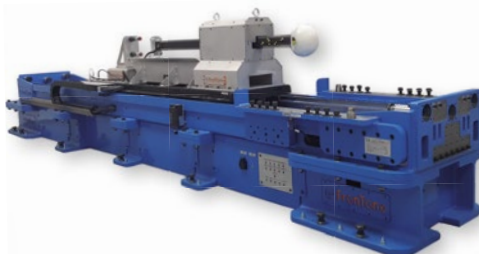
Airbag Component Test Rig for various airbag- and steering column tests
