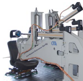
Seat back and head restraint performance test rig
