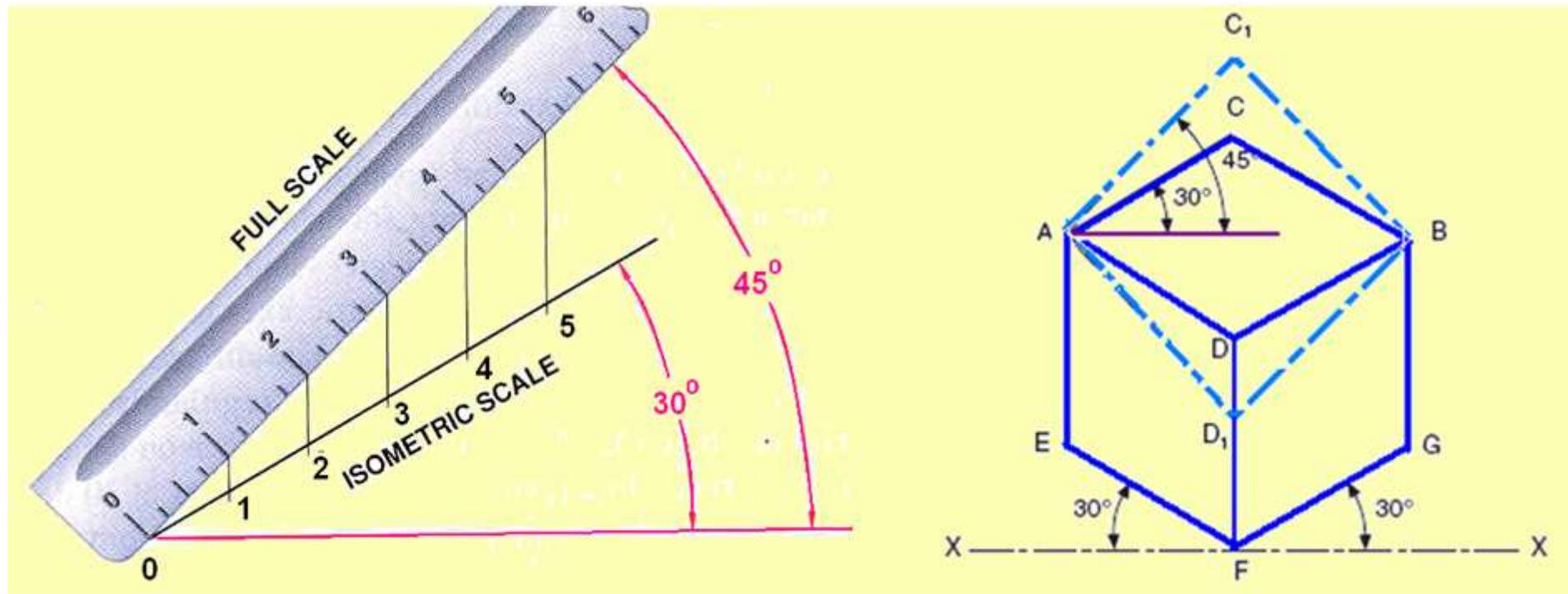
$$\text{Isometric scale} = \left( \frac{\text{Isometric length}}{\text{True length}} \right) = \frac{\cos 45^\circ}{\cos 30^\circ} = \frac{1}{\sqrt{2}} + \frac{\sqrt{3}}{2} = 0.8165$$
