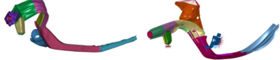
Full Vehicle Model Dynamic impact analysis
