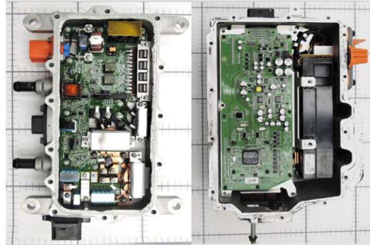
Figure 67: Cutaway of a DC/DC converter (left) and inverter (right)
