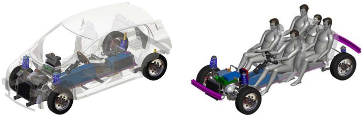
Figure 2-2: Powertrain Component and Passenger Packaging
