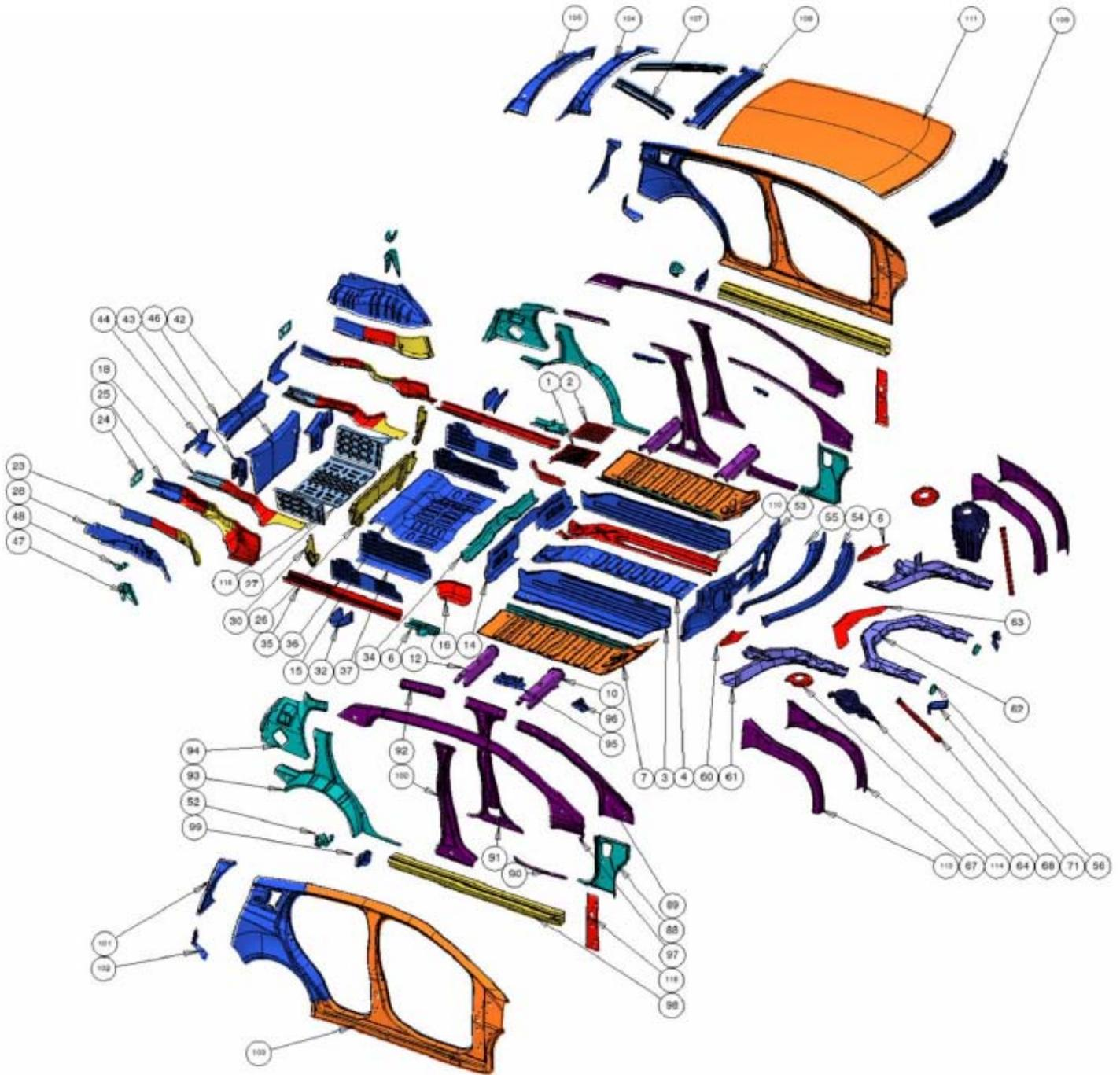
Figure A3-1: BEV Exploded View
