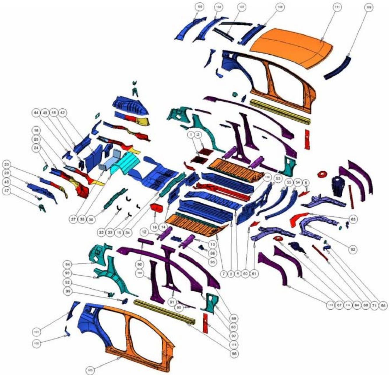
**Figure A4-1: FSV-1 PHEV<sub>20</sub> Exploded View**
