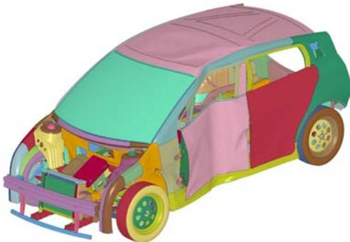
**Figure 3-23: FMVSS 216-a Roof Crush Deformed passenger side-roof structure at rigid plate movement 127 mm**
