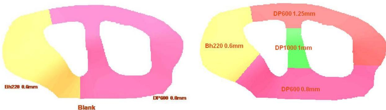
**Figure 3-31: Body Side Outer Two-Piece Option (left) and Four-Piece Option (right)**
