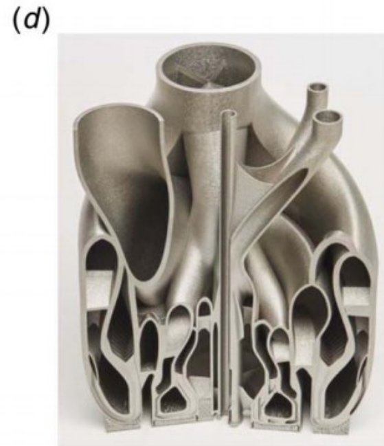
Fig. 17 Examples of additively manufactured parts with complex architectures: (a) aircraft duct consolidated from many parts into a single, complex part (reprinted by permission from Springer, [79]), (b) additively manufactured screen for a downhole drilling application [80], (c) mathematically inspired artwork (courtesy of Bathsheba Grossman), and (d) a burner with organically shaped flow channels (courtesy of Siemens)
