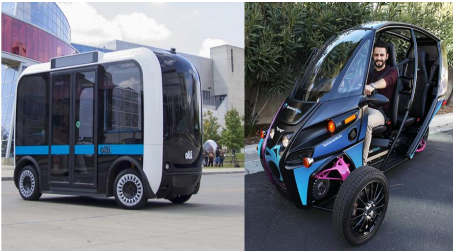
Electric shuttle Olli (left) and Arcimoto's FUV (right) feature 3D-printed components. The use of 3D printing helped to reduce the weight of the vehicles. [Image credits: Local Motors, Arcimoto]
