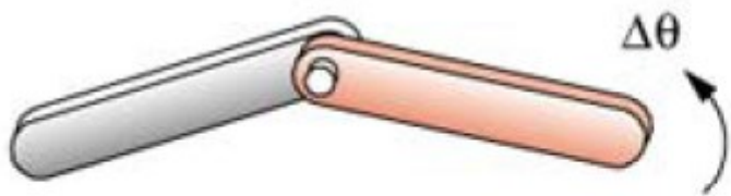
Rotating full pin (R) joint (form closed) pin (or revolute) joint
