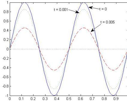
$$u(x, t) = G(x)H(t) \rightarrow \frac{\partial u}{\partial t} = \frac{\partial^2 u}{\partial x^2} \rightarrow G \frac{dH}{dt} = H \frac{d^2G}{dx^2} \rightarrow \frac{1}{G} \frac{d^2G}{dx^2} = \frac{1}{H} \frac{dH}{dt} = (\text{constant}) = -k^2 \quad (5 \text{ pts})$$
