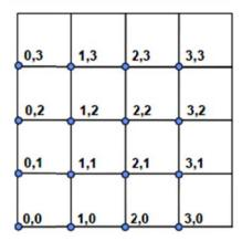
Simple Laplacians are used for all interior nodes. Balances for the edges must take insulation into account. For example, node 1,0 is modeled as
