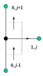
A flux balance around the node can be written as (note  $\Delta x = \Delta y = h$ )
