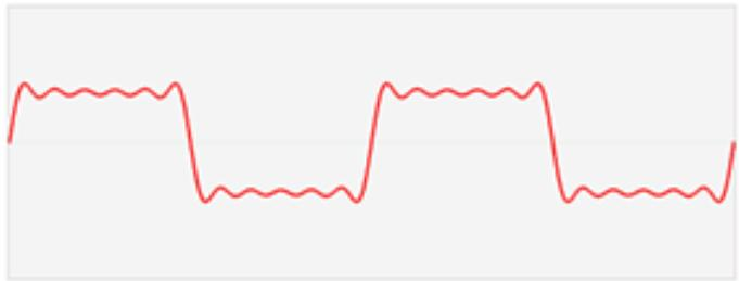
$$\begin{cases} F(x) = \sum_{n=-\infty}^{\infty} c_n e^{inx} = c_0 + c_1 e^{ix} + c_{-1} e^{-ix} + \dots \\ \int_{-\pi}^{\pi} F(x) e^{-ikx} dx = 2\pi c_k \rightarrow c_k = \frac{1}{2\pi} \int_{-\pi}^{\pi} F(x) e^{-ikx} dx \end{cases}$$
