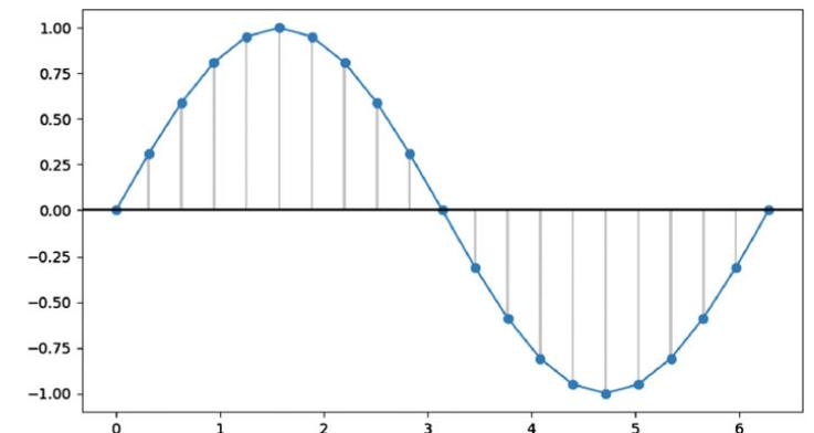
$$\begin{cases} g(t) = a_0 + \sum_{i=1}^n a_i \sin(i\omega t) + \sum_{i=1}^n b_i \cos(i\omega t) \\ a_n = \frac{\omega}{\pi} \int_0^{\frac{2\pi}{\omega}} g(t) \sin(n\omega t) dt \\ b_n = \frac{\omega}{\pi} \int_0^{\frac{2\pi}{\omega}} g(t) \cos(n\omega t) dt \end{cases} \rightarrow \begin{cases} g(t) = A_0 + \sum_{i=1}^n A_i \sin(i\omega t + \theta_i) \\ A_n^2 = a_n^2 + b_n^2 \\ \theta_n = \tan^{-1} \left( \frac{b_n}{a_n} \right) \end{cases}$$
