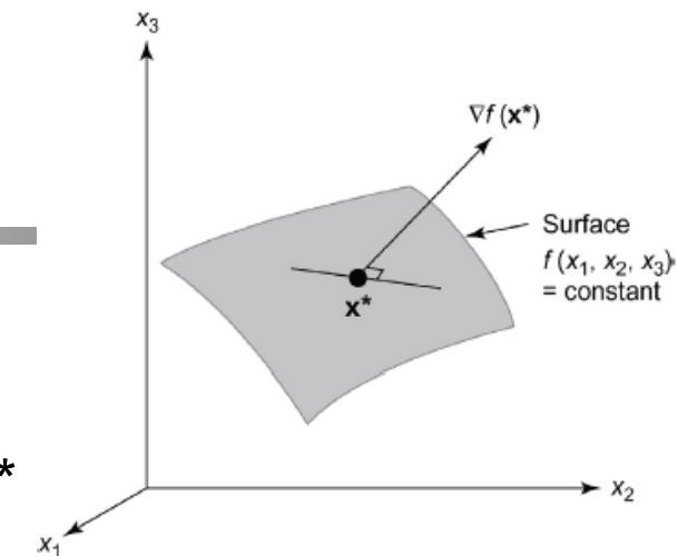
$$\nabla f(\mathbf{x}^*) = \frac{\partial f(\mathbf{x}^*)}{\partial \mathbf{x}} = \text{grad } f(\mathbf{x}^*) = \left[ \frac{\partial f(\mathbf{x}^*)}{\partial x_1} \quad \dots \quad \frac{\partial f(\mathbf{x}^*)}{\partial x_n} \right]^T$$
