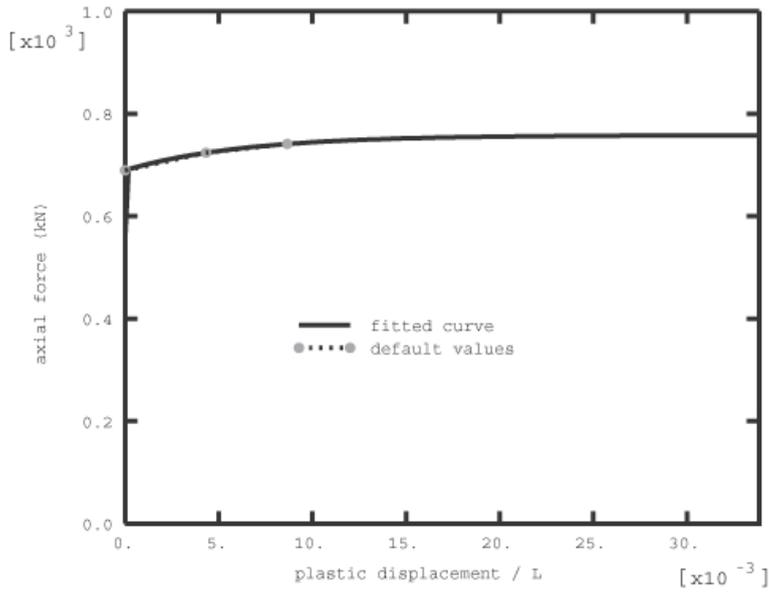
Figure 3. Default hardening response for bending moments in a typical element with PIPE cross-section (element 7 in the model).
