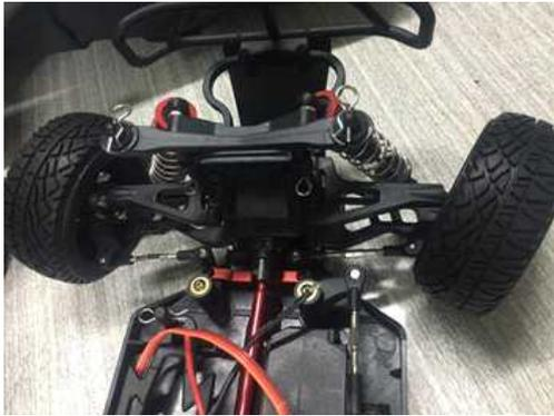
Photo. 1 Steering structure of model car
