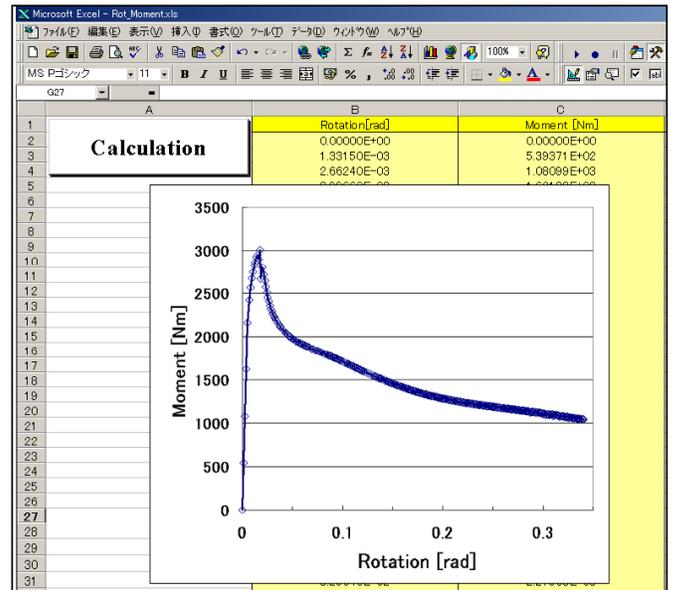
Figure 12. Moment-rotation angle characteristic automatically obtained by Excel using a macro language
