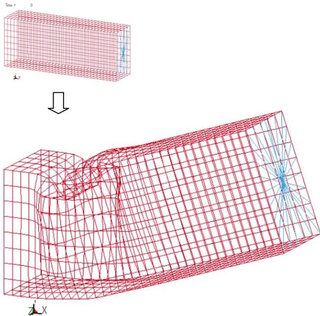
Figure 11. Deformation shape obtained by collapse analysis of cantilever using LS-DYNA
