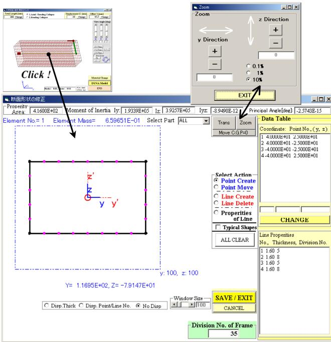
Figure 4. Sub frame to create cross-sectional shape
