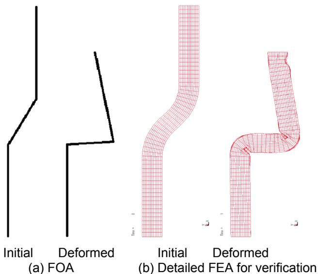
Figure 17. Deformed shapes obtained by FOA and detailed FEA for verification
