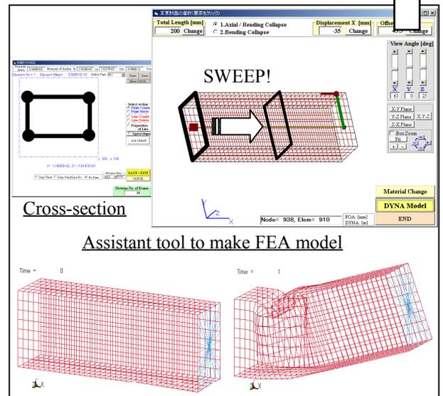
(c) Collapse analysis-using LS-DYNA for bending part
