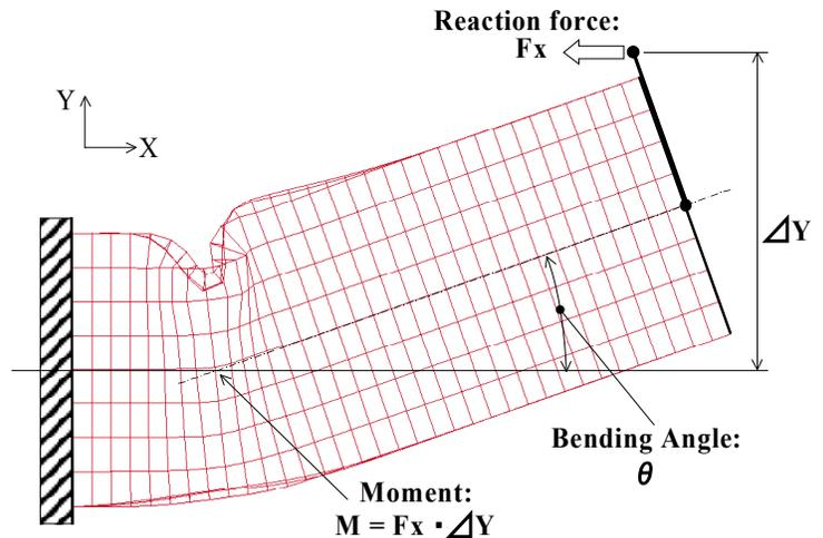
Figure 6. Relationship between applied moment  $M$  and deformed shape
