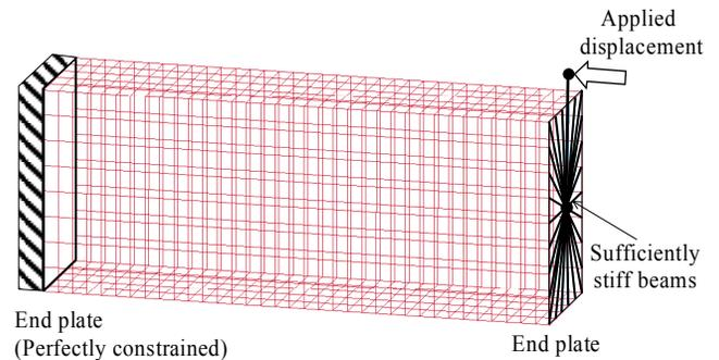
(a) Loading condition of combined axial force and bending moment of cantilever
