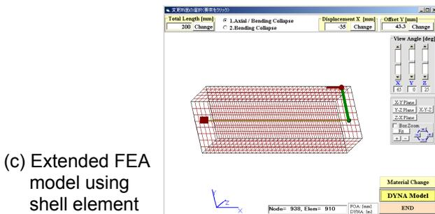
(c) Extended FEA model using shell element
