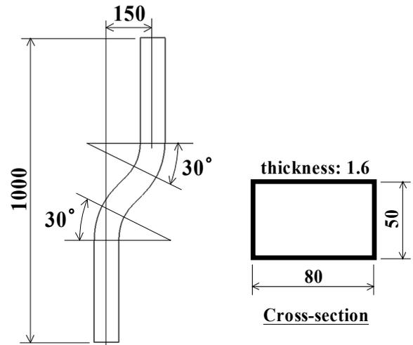
Figure 8. Dimensions of structural member for example
