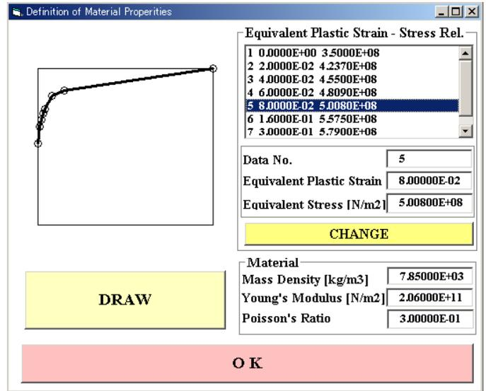
Figure 5. Sub frame to input material characteristic
