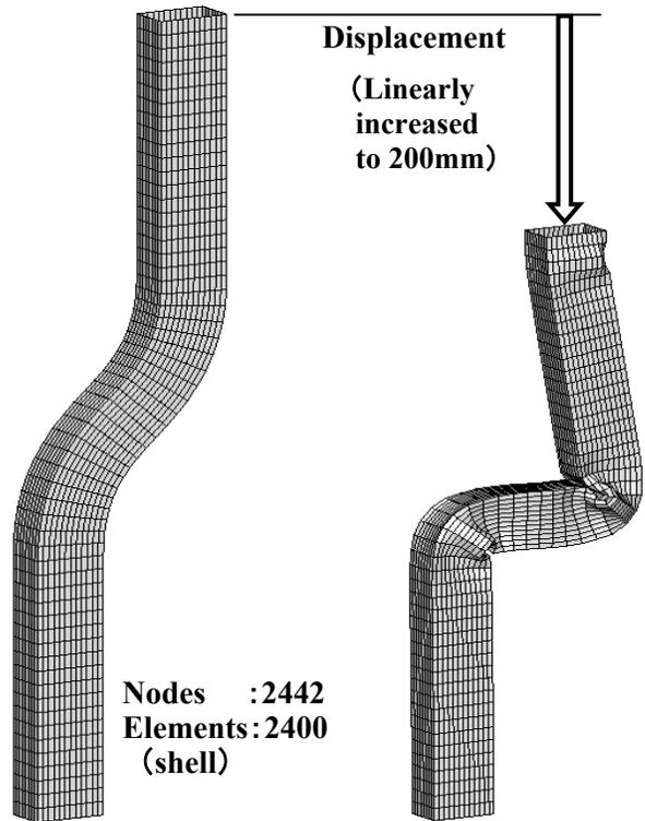
Figure 16. Detailed FEA model using shell element for verification
