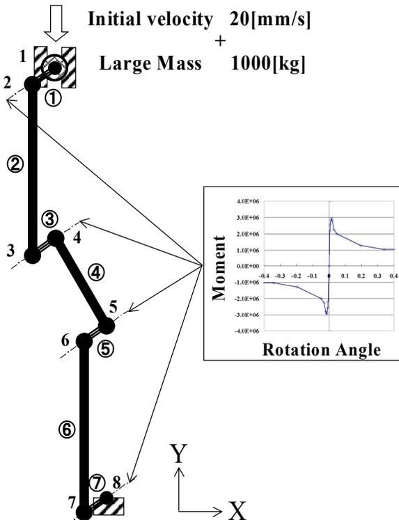
Figure 15. Illustration of FEA model for in-house software
