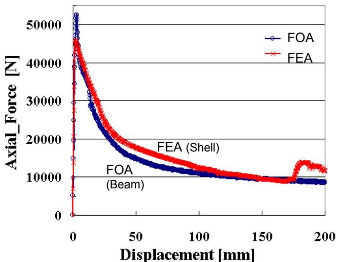
Figure 18. Relationship between reaction force ( $F_y$ ) and displacement ( $\delta Y$ ) of moving point obtained by FOA (Beam) and detailed FEA (Shell) for verification
