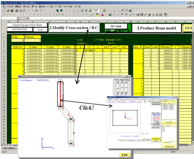
Figure 14. Excel sheet for FEA model using beam element of structural member
