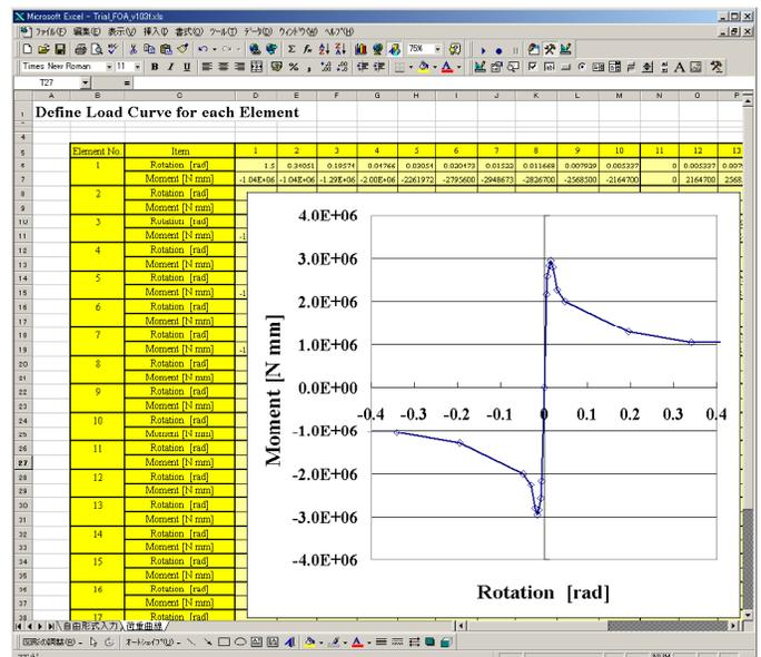
Figure 13. Moment-rotation angle characteristic inputted into Excel sheet by reducing redundant data
