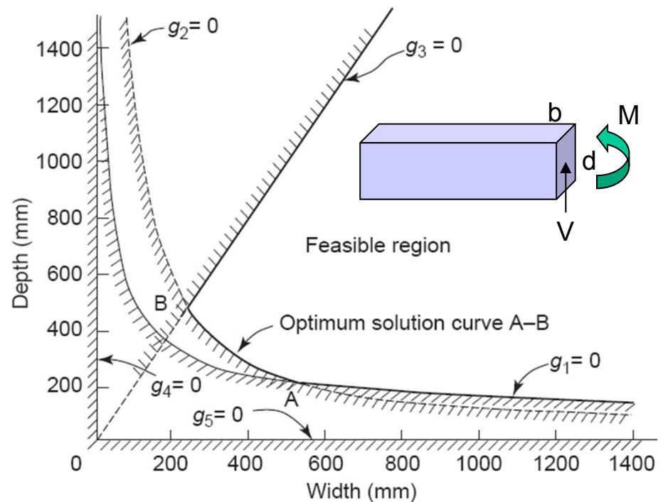
$$b = 237 \text{ mm}, d = 474 \text{ mm} @ \text{point B}$$
