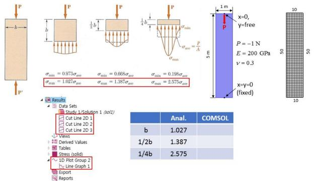
4. [Stress concentration] The flat bar with a hole has a thickness of 1 m. The dimensions and boundary conditions are shown in the following figure.
