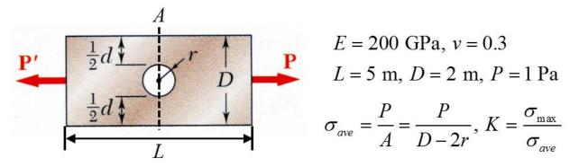
1) Compute the maximum normal stress(solid.sx) with r = 0.5 m. Construct a quarter model and set the mesh options as shown in the following figure. (15 pts)
