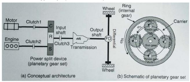
Inertia/mass :  $J_{engine} = 0.2 \text{ kg} \cdot \text{m}^2$ ,  $J_{motor} = 0.05 \text{ kg} \cdot \text{m}^2$ ,  $J_{wheel} = 1 \text{ kg} \cdot \text{m}^2$  (sum of wheels),  $m_{body} = 1,500 \text{ kg}$
