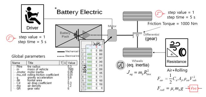
5. [AMESim] The purpose of an EV shown in the figure is to evaluate 0-100 km/h acceleration time and maximum speed.
