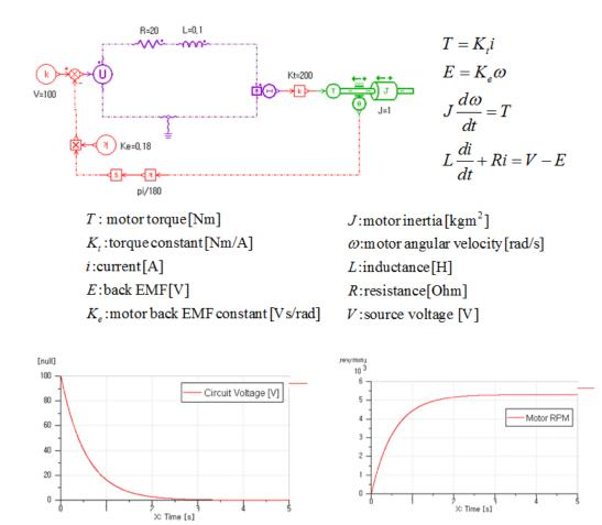
4. [Simulink] Consider this electric motor circuit model by AMESim. The parameter values are indicated on the diagram.
