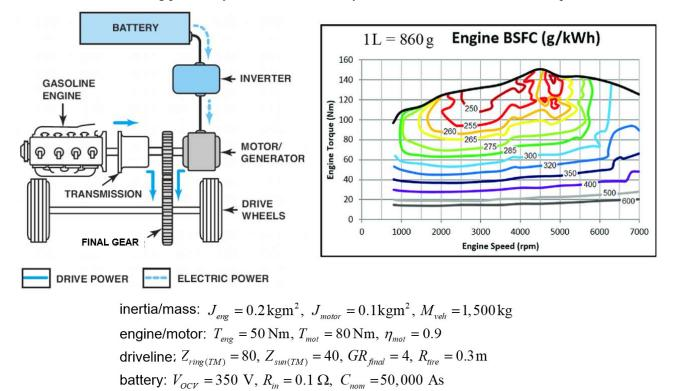
6. Consider the following parallel hybrid electric vehicle system. Be sure to check the units of parameter values.
