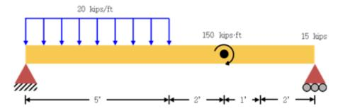
Using singularity function the displacement along the beam can be expressed by the equation.
