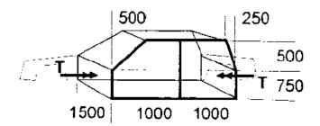
4. Consider the impact of the vehicle( $M_2$ ) by a moving barrier( $M_1$ ). We can model each as a point mass with the impact being perfectly plastic. In this linear model, we are looking at motions lateral to the vehicle and will consider the lateral component of the barrier velocity as the initial impact velocity.
