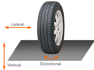
Fig. 4 Vertical, lateral and distortional stiffness of a tire
