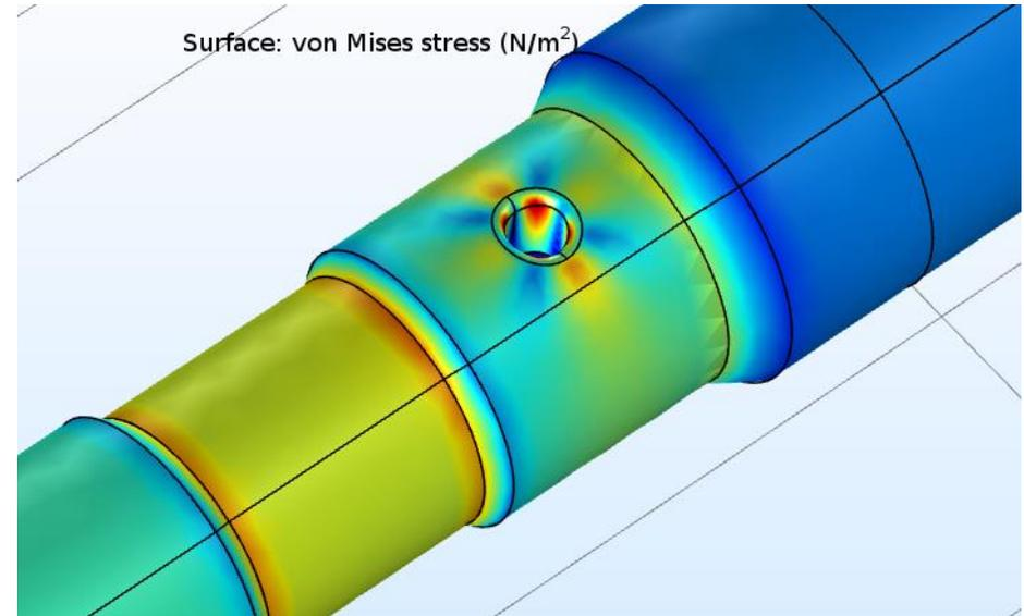
Complete mesh consists of 160668 domain elements, 27206 boundary elements, and 3134 edge elements.
