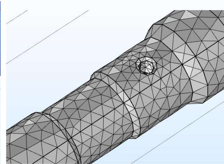
Used linear geometry shape in 19 mesh elements to avoid inverted curved elements.
