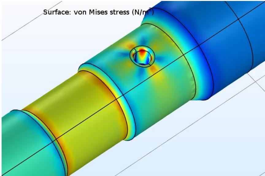
Used linear geometry shape in 28 mesh elements to avoid inverted curved elements.
