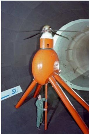
Figure 10: The ONERA-DLR ERATO rotor mounted in the SIMA 8 m Ø closed test section.
