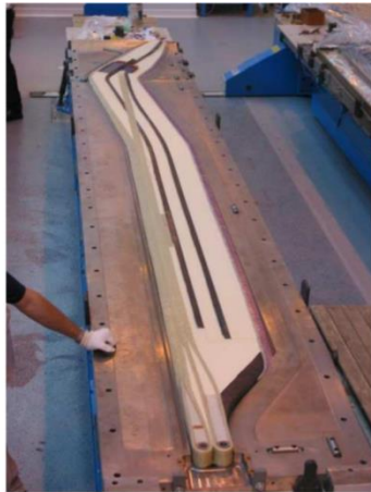
Figure 33: Molded structure of the experimental Blue Edge™ blade.
