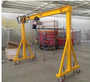
small overhead crane (0.5t)
